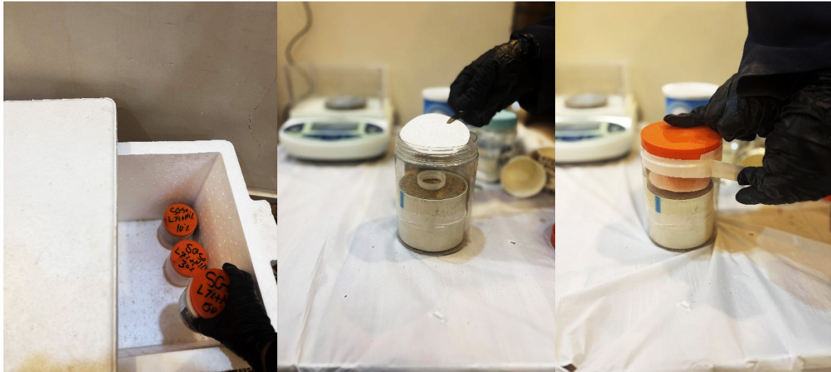
Figure 3. Steps of conducting total suction by filter paper
