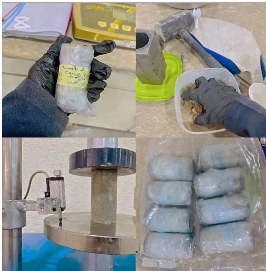
Figure 7. Steps for conducting a compressive strength test
