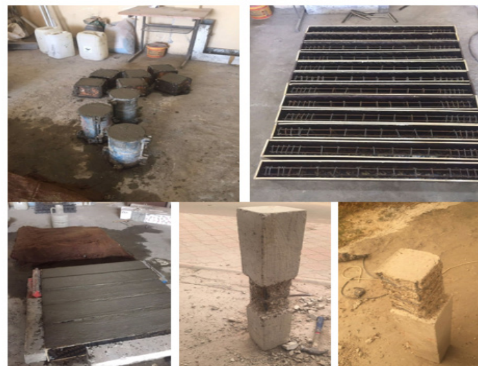
Figure 2. Casting and preparation of the columns and control specimens for test
