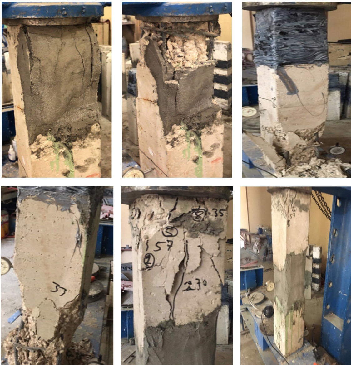
Figure 9. Cracks pattern for columns
