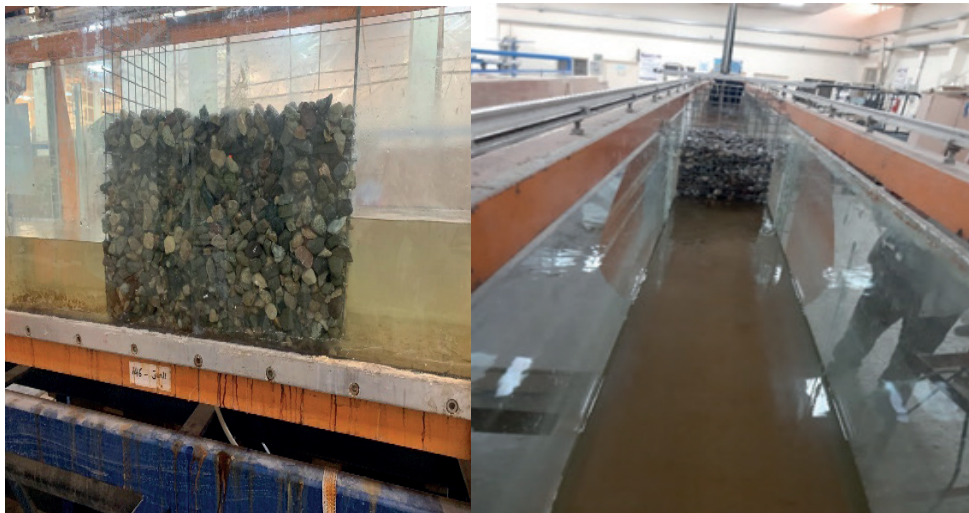
Figure 2. Self-Spillway dam model
