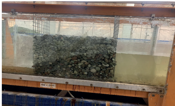
Figure 5. Hydraulic gradient through Self-Spillway dam at the maximum given discharge
