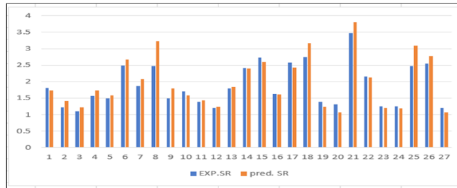
Figure 8. Variance in Experimental and Predication Values of the Process Parameters for the Surface Roughness
