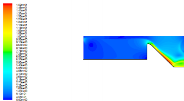
Figure 5. Velocity Distribution over Ogee Spillway
