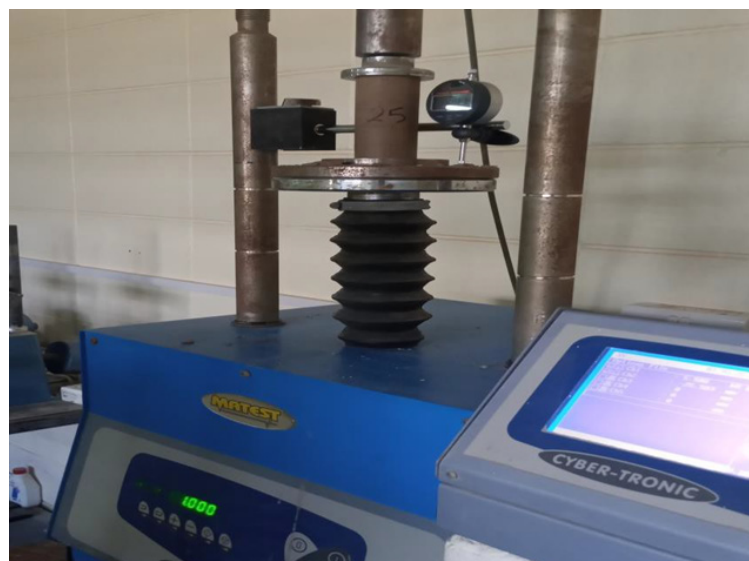
Figure 2. Unconfined Compressive Strength test
