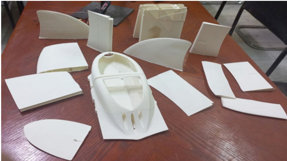
Figure 8. The use of LW-PLA material in the manufacture of the E-VTOL aircraft frame
