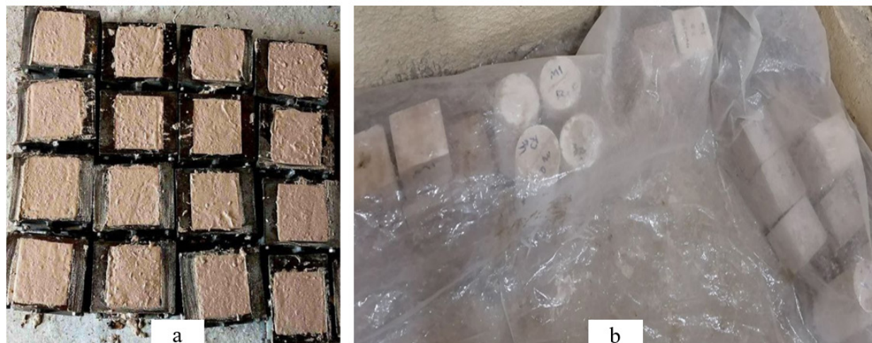
Figure 2. Preparation of SCGPC samples: (a) cast specimens (b) Casting samples are covered in plastic until the day of testing
