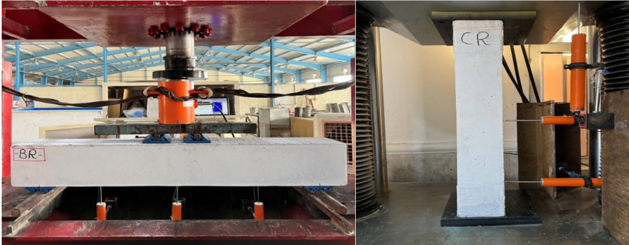
Figure 4. Test setup for beam and column
