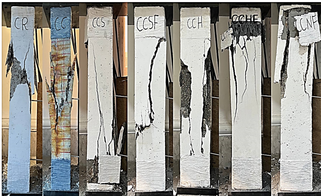
Figure 8. Modes of cracking in RC columns using different types of concrete
