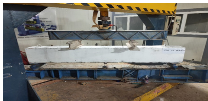
Figure 2. Tested device of beams
