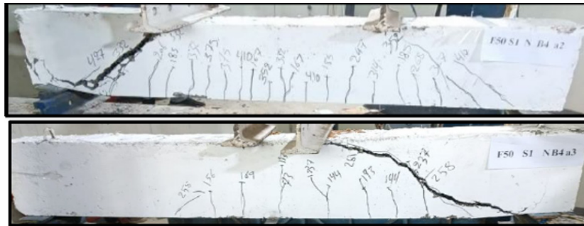
Figure 13. Crack pattern of test specimens under effect of shear span to effective depth ratio with steel fiber
