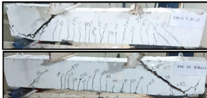
Figure 16. Crack pattern of test specimens under effect of type of aggregate with steel fiber
