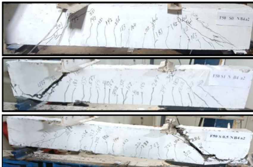
Figure 7. Crack patterns of test specimens under effect of volume fraction of steel fiber
