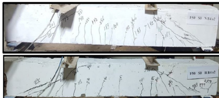
Figure 17. Crack pattern of test specimens under effect of type of aggregate without steel fiber
