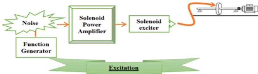
Figure 6. Excitation side of random vibration
