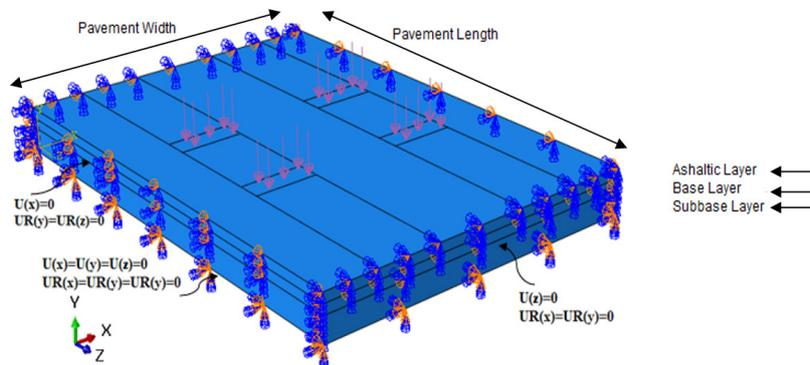
Figure 7. Pavement geometry and boundary condition of models
