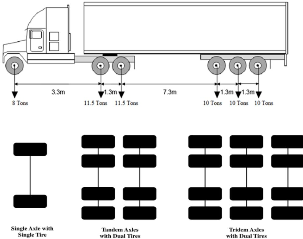
Figure 5. Axle loads used in models for truck type 3-S3
