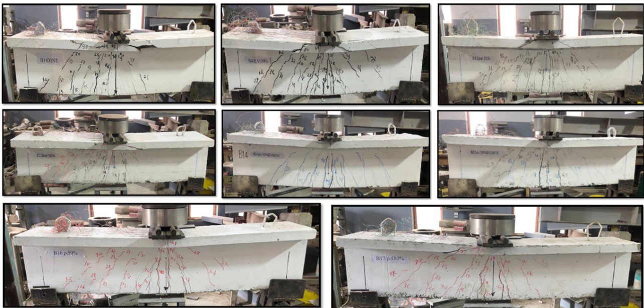
Figure 11. Cracks patterns with the applied load and mode failure
