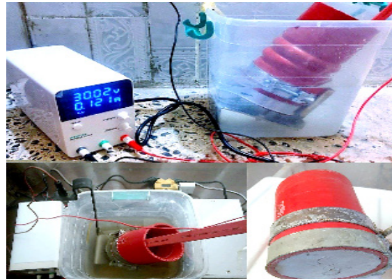
Figure 7. Rapid chloride migration test
