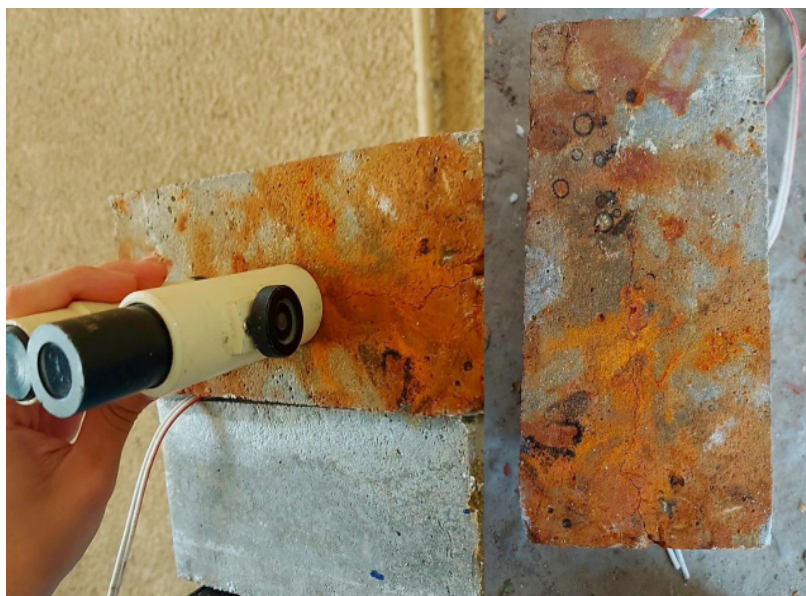
Figure 18. Method of measuring the crack width
