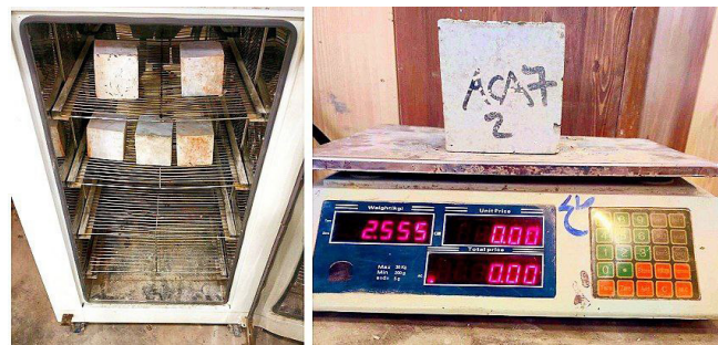
Figure 5. Water absorption test
