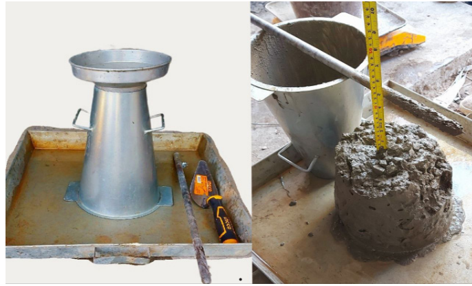
Figure 3. Slump flow test
