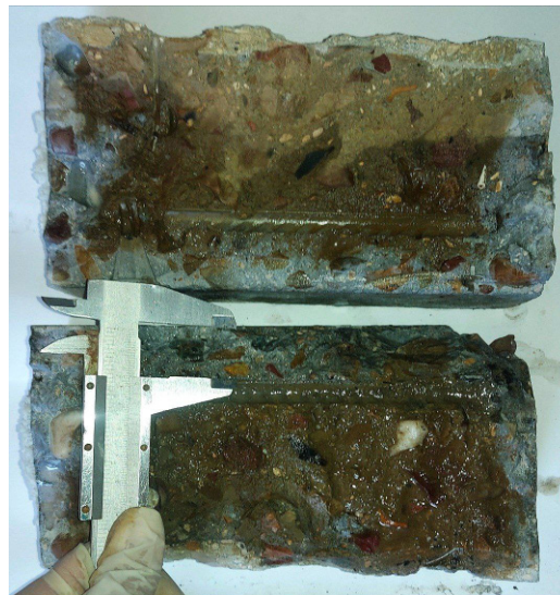
Figure 8. Chloride penetration test
